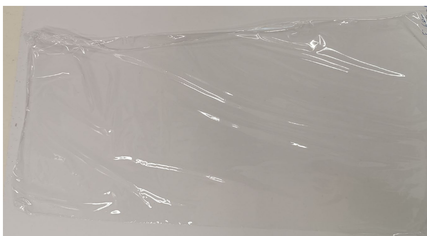
Figure 1: Symmetric dense membrane obtained from the 16.5%TPU-83.5%DMF casting solution.
