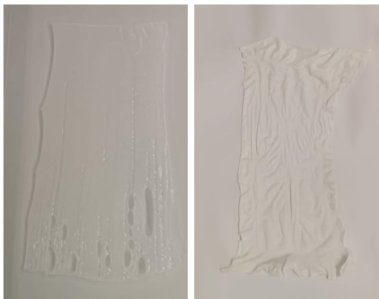
Figure 4: (Left) Integrally asymmetric MMM obtained from the nanoparticle dispersion with air bubbles present; (Right) Integrally asymmetric MMM obtained from the nanoparticle dispersion with no air bubbles.
