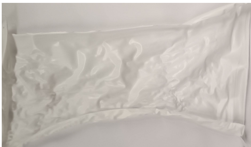
Figure 2: Integrally asymmetric membrane obtained from the 13.9%TPU-70.6%DMF-15.5%ACET casting solution.
